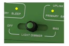
For optional status panels and optional HD camera IR illuminator, a light dimmer control can be set with a mechanical lever and reliable friction lock, to ensure that the illumination intensity is adjusted to a level suitable for the operational environment, from absolute zero light to bright light in 16 steps.
