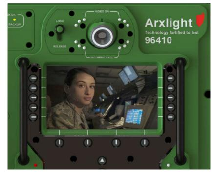
A mechanical shutter is included in video camera lens, that effectively closes the camera lens when video is not used, securing unauthorized video viewing. VIDEO ON status shows open shutter.
